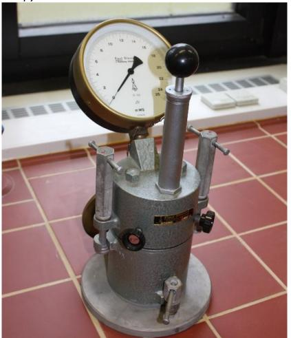
DIN EN ISO 17892-3: Determination of particle density
