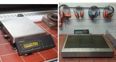
Electronic scales with a resolution of: 0,0005 g 0,01 g 0,1 g 1,0 g
