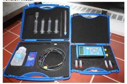
A tension meter is a device used to measure soil water tension or matrix potential. Measuring range:
