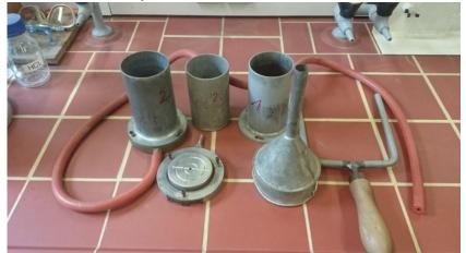
DIN 18126 Determination of density of non-cohesive soils for maximum and minimum compactness
