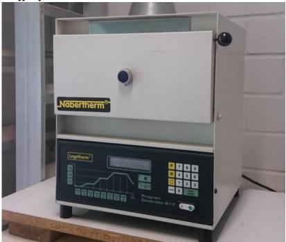
DIN 18128 Determination of ignition loss
