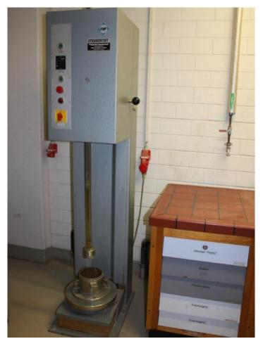
Proctor device for performing Proctor tests DIN 18127 with Proctor molds: 100mm, 150mm, 250mm diameter
