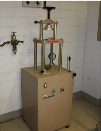
For press soil samples and asphalt bodies D = 96 mm and D = 150 mm out with equipment for undisturbed sampling
