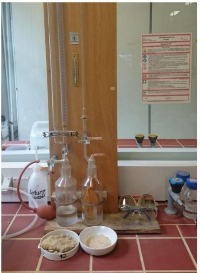
Test: DIN 18129 Determination of lime content
