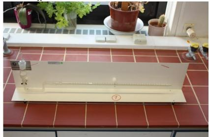
Test: DIN 18132 Determination of water absorption
