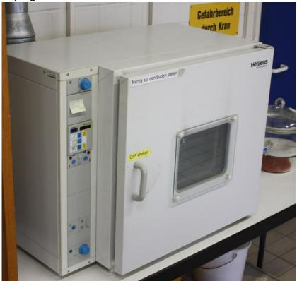
Convection drying ovens with electronic temperature control
