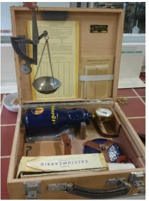
Determining Water Content in Soil within Calcium Carbide Method
