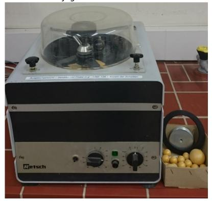
For dry and wet grinding organic and inorganic substances Grinding fineness approx. 1  $\mu m$
