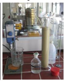
Areometer equipment: electric suspension mixer, glass cylinder D = 6 cm, plastic stoppers, electronic thermometer; 6 sieves D = 12 cm, mash from 0,06 mm to 2 mm for the hand sieving
