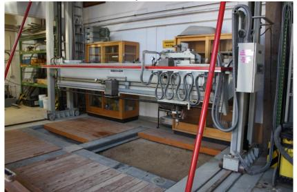
With this device, tensile and compressive loads (up to 160 kN) can be applied statically and cyclically via control electronics. In our test pit (4 x 4 m²), which is up to 6 m deep, model tests can also be carried out
